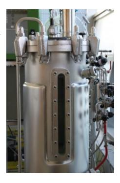
Each bioreactor feeds into the next. The train is a continuation of the scale up process that begins with the inoculum preparation stage and ends usually with the harvesting process in the largest bioreactor.
