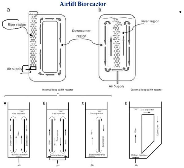
An ALR, or airlift reactor, is a pneumatically-driven bioreactor especially suitable for large-scale culture of immobilized plant cells.
