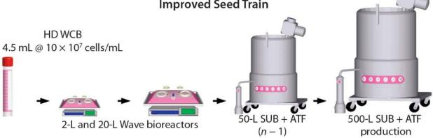
The illustration compares a novel seed-train process using HD cell banking, disposable Wave bioreactors, and Refine Technology's Alternating Tangential Flow (ATF) perfusion cell-culture technologies over a conventional one. An example of this process for a 500-L production perfusion bioreactor with a conventional seed-train process.
