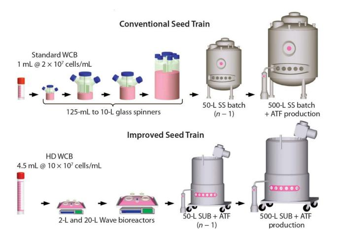
The illustration compares a novel seed-train process using HD cell banking, disposable Wave bioreactors, and Refine Technology's Alternating Tangential Flow (ATF) perfusion cell-culture technologies over a conventional one. An example of this process for a 500-L production perfusion bioreactor with a conventional seed-train process.
